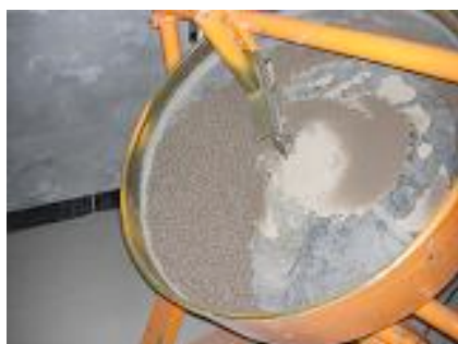
Figure 9. Making Clay Dumpling. SOMRE Treated Seeds are Inside.
